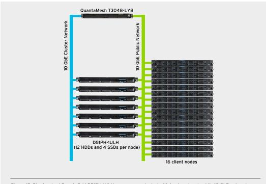
Figure 12. Six standard QuantaGrid D51PH-1ULH servers were tested with back end and public 10 GbE networks.
