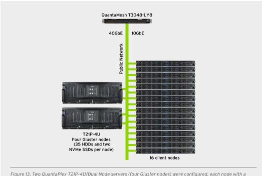
Figure 13. Two QuantaPlex T21P-4U/Dual Node servers (four Gluster nodes) were configured, each node with a 40 GbE interface, with the configuration driven by 16 client nodes.
