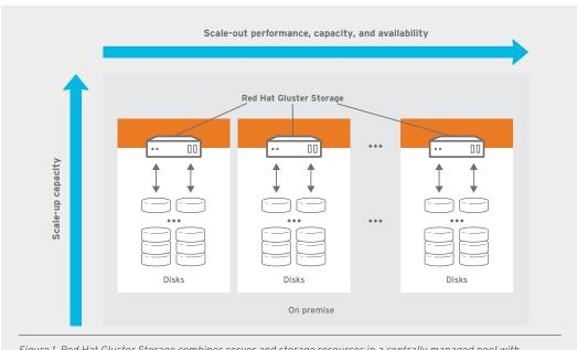
Figure 1. Red Hat Gluster Storage combines server and storage resources in a centrally managed pool with independent capacity and performance scalability.
